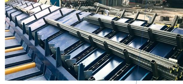
Chain conveyor system which creates buffer between shearline and double bender.
