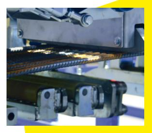
Accurate, quick and safe selecting and counting of rebar through innovative design with servo drive system.
