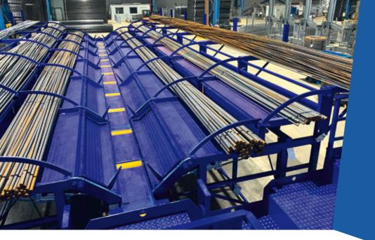
Solid storage rack with multiple levels to store different rebar diameters. The surface of the rack is completely closed with tear plate for safe operation. The row of hooks on both sides of the infeed conveyor provide possibility to preload bars already during the previous cutting cycle.
