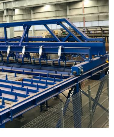
Safest way of loading of new bundles through automatic bundle loading system. Supply of new bundles into the loading system possible by overhead crane or by conveyor.
