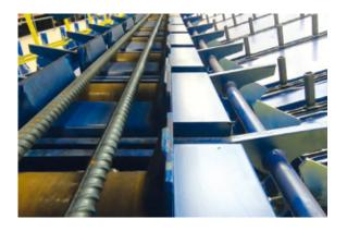
▲ After the infeed-cutting process, bars are dropped on the distribution roller conveyor.
