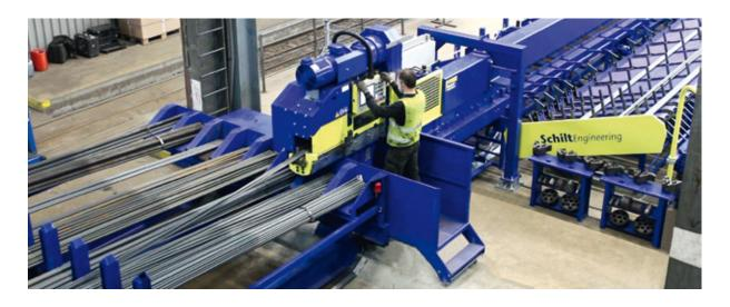
A Ergonomic workplace design. Easy inlay of bars and safe handling.
